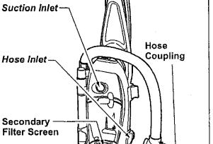
Unplug vacuum. Remove hose coupling and check hose coupling and hose inlet for clogs. Check suction inlet and secondary filter screen for clogs.
